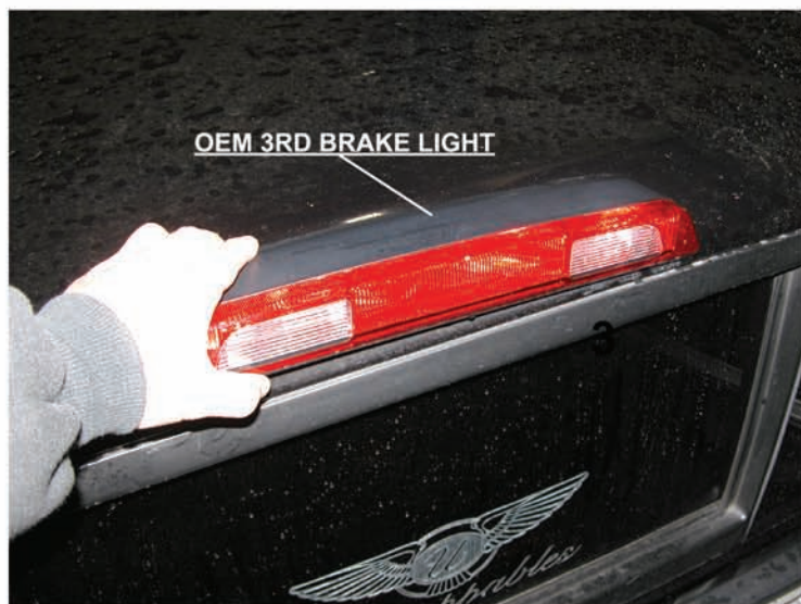
5. Pull out the OEM 3rd brake light
