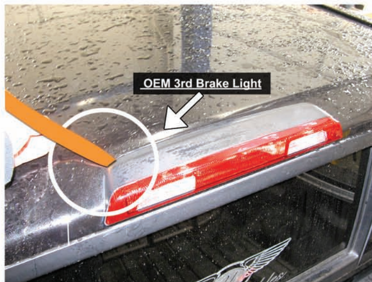
4. Carefully loosen the OEM 3rd brake light from the roof
