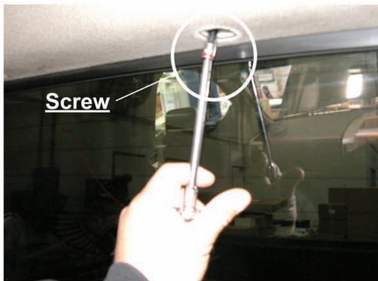
10. Reinstall both screws inside the ceiling of the vehicle
