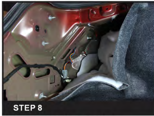
STEP 8 Nuts and connector connected
