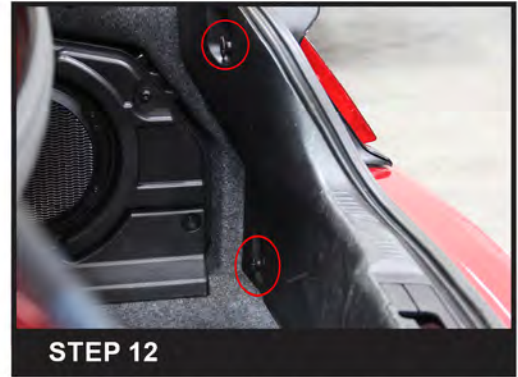
STEP 12 Install four retainers that hold the trim panel, two on each side
