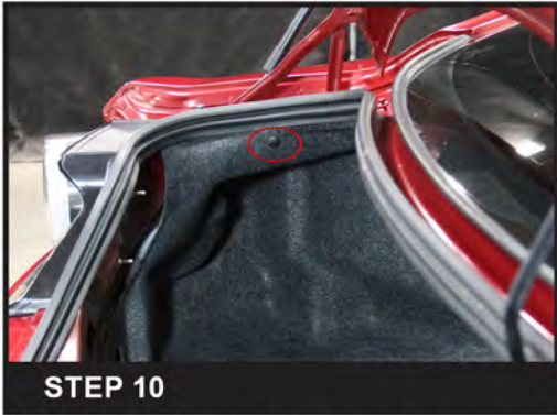
STEP 10 Reinstall the push pin for both side
