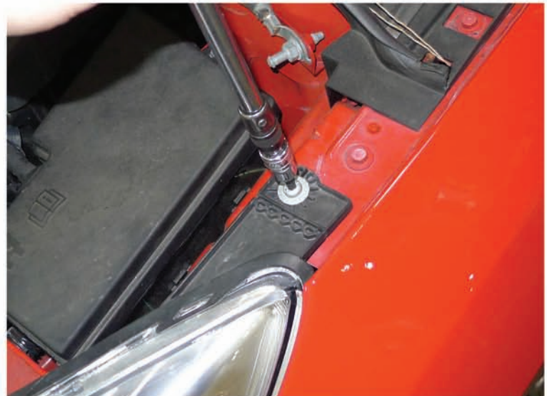
4. Remove the (2) T30 bolts
