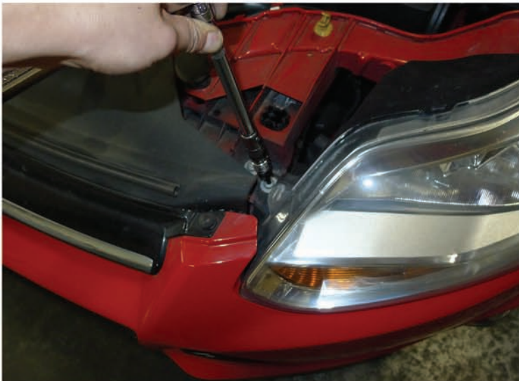
3. Remove the (2) T30 bolts
