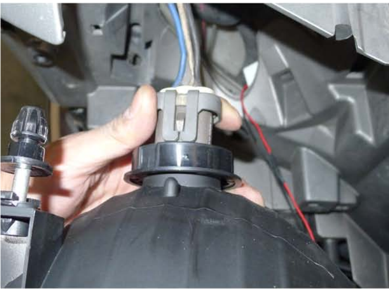
11. Install the headlight bulb and connect the headlight harness to the new headlight Please see the "HALO and L. E. D. head lights installation instructions" If your head lights don't have HALO and L.E.D. You can skip the installation instruction.
