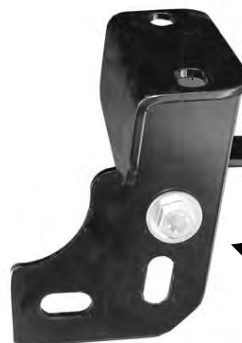
(Fig 3) Driver side Support Bracket in "no Tow Hook" position
