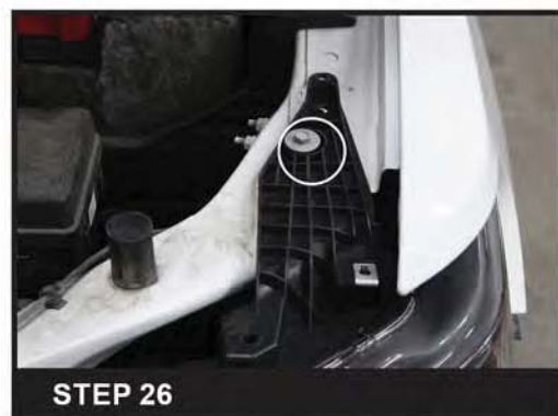
STEP 26 Reinstall the 10mm headlight bolt at the top of the headlight
