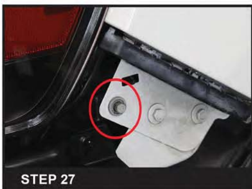
STEP 27 Reinstall the 10mm headlight bolt at the bottom of the headlight
