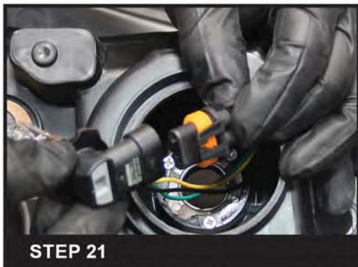
STEP 21 Reinstall the high beam light bulb to the new headlight housing
