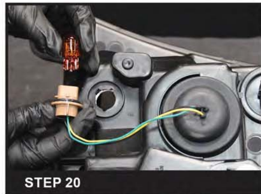
STEP 20 Reinstall the signal light bulb to the new headlight housing signal light socket
