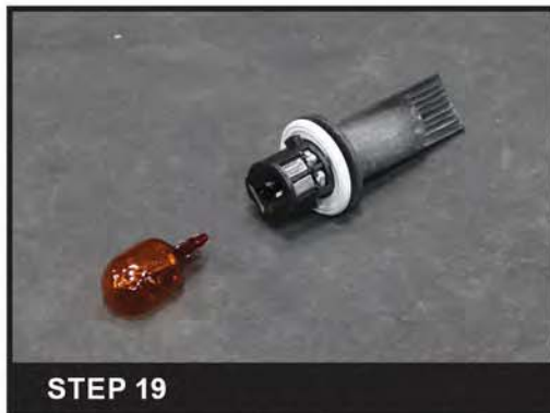
STEP 19 Remove the signal light bulb from the signal light socket
