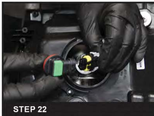
STEP 22 Reinstall the low beam light bulb to the new headlight housing
