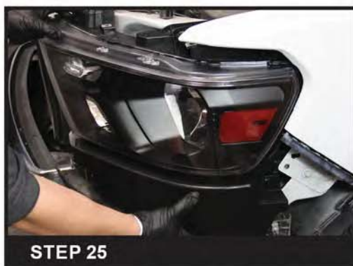
STEP 25 Seat the new headlight assembly in place
