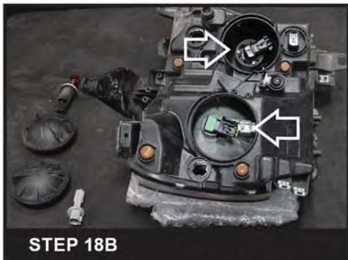
STEP 18B Remove the high beam and the low beam light bulbs from the factory headlight housing
