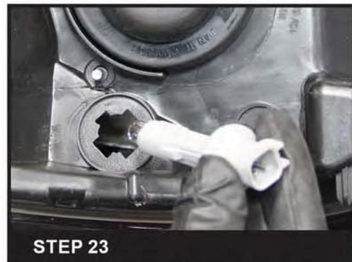
STEP 23 Reinstall the parking light socket to the new headlight housing
