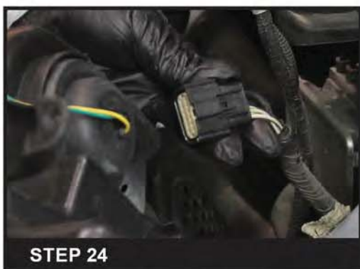
STEP 24 Connect the headlight harness
