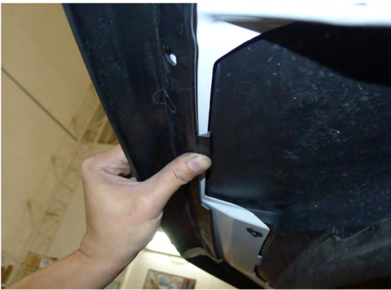
5. Hook the locating tab against the edge of the bumper.
