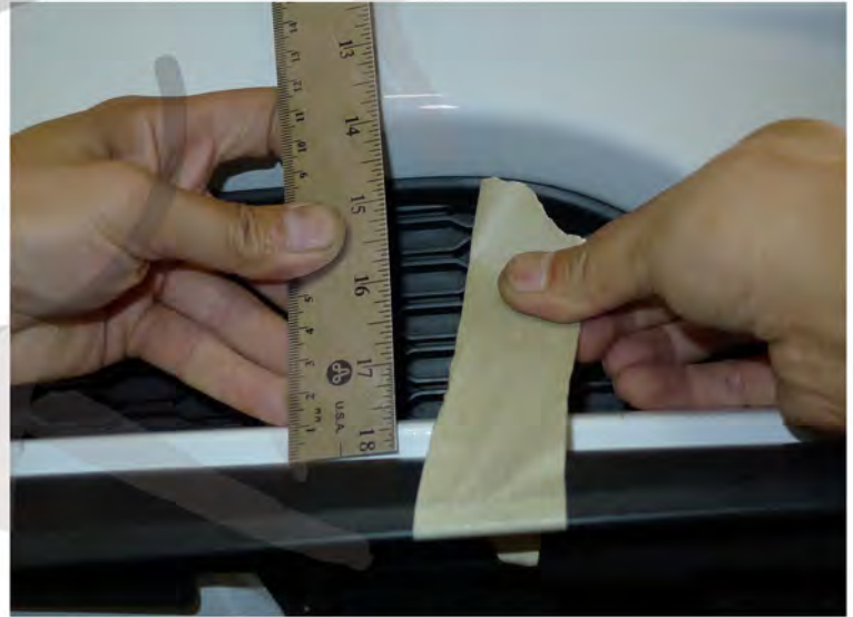
2. Temporarily tape the lip into the position
