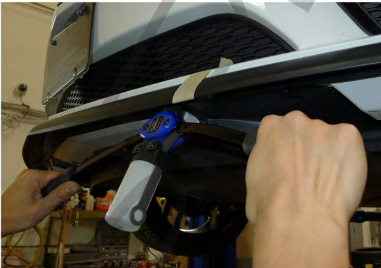
10. Install an ssecure front lip using 11 plastic rivets
