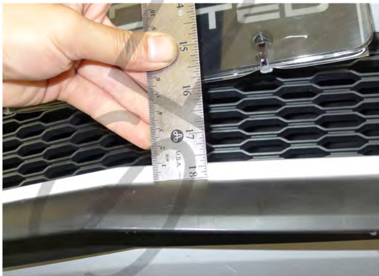
3. Measure the distance between the lip and leading the edge of the lower bumper
