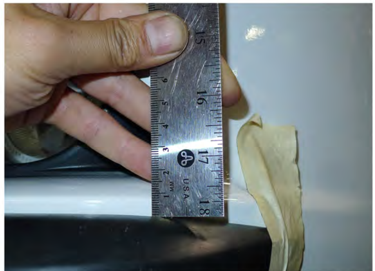
4. Measure and position the lip with even spacing from the leading edge of the bumper
