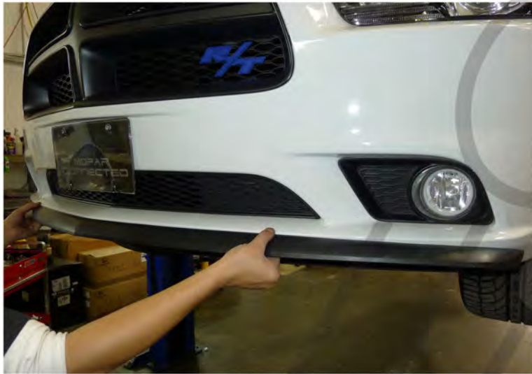
1. Place the front lip up against the bottom edge of the front bumper
