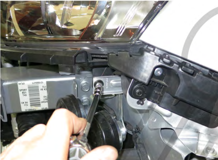
25. Tighten the 7mm bolt
