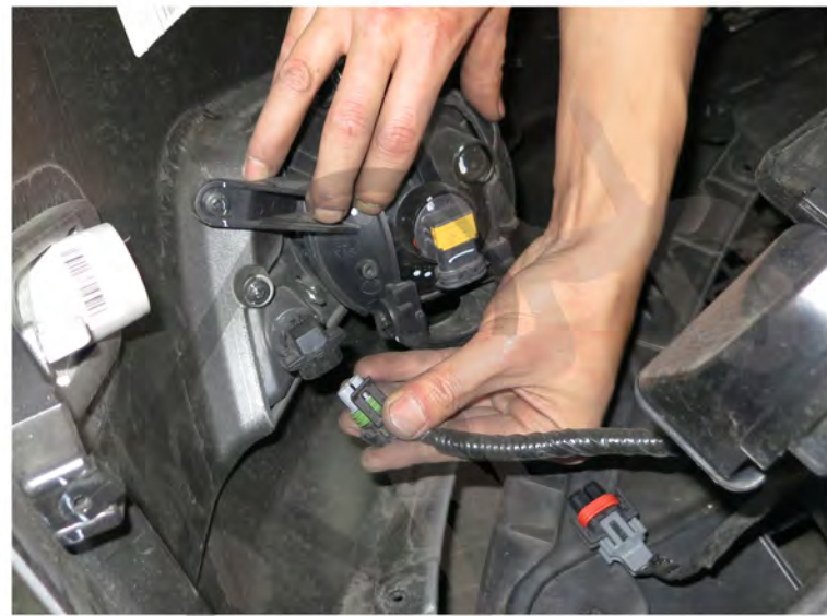
12. Disconnect the air temp sensor harness
