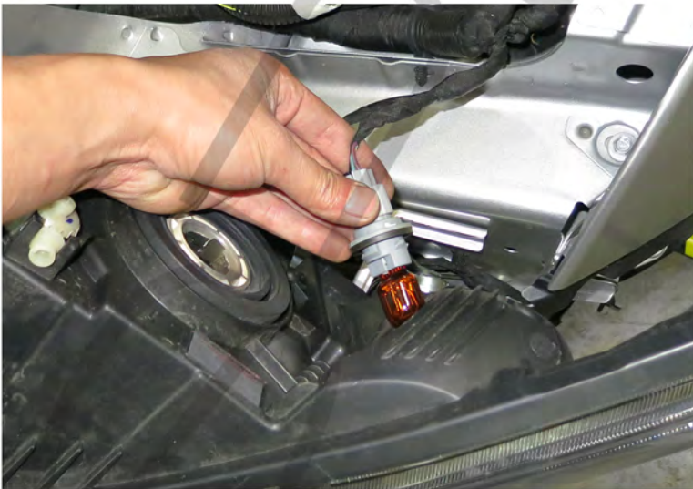
21. Remove the signal light bulb
