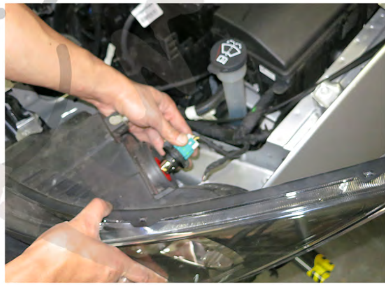
20. Remove the headlight bulb
