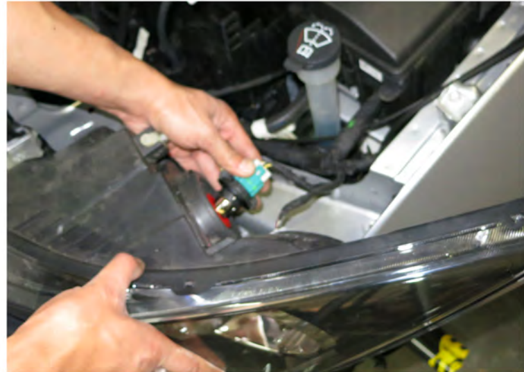
22. Install the headlight into the new headlight
