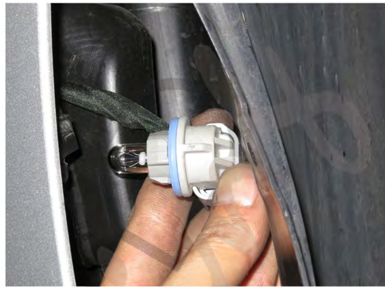
6. Remove the bumper light socket
