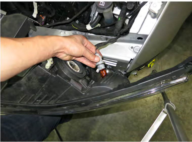
23. Install headlight harness
