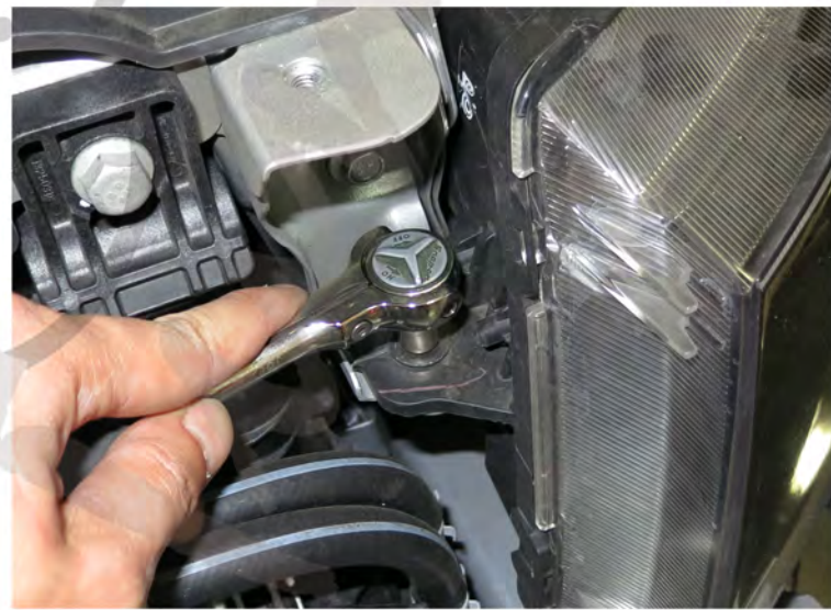
14. Remove the 7mm bolt
