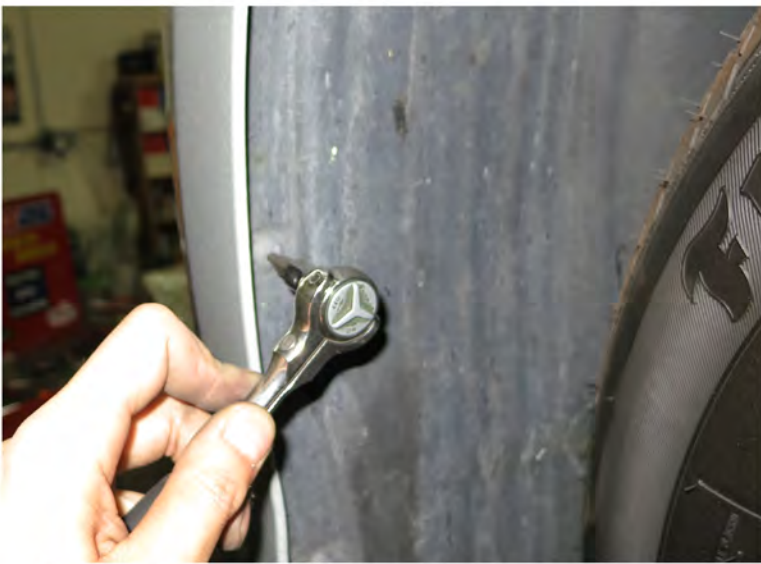
5. Remove the (3) T30 screws
