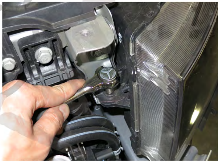
26. Tighten the 7mm bolt
