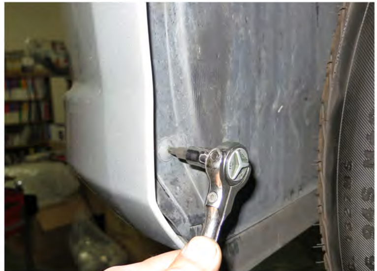
4. Remove the (3) T20 screws
