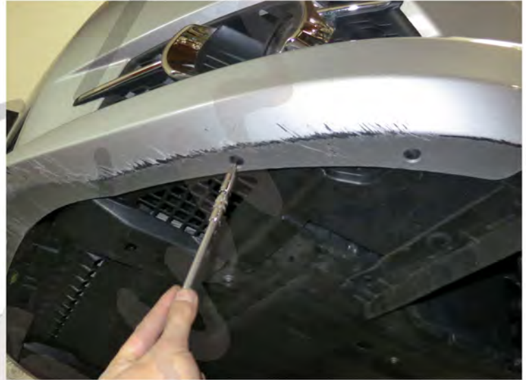
2. Remove the (8) T20 screws
