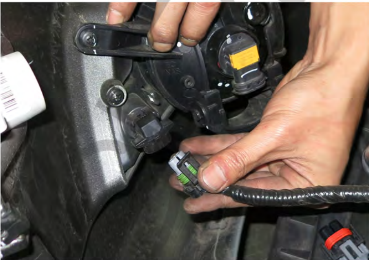
27. Connect air temp sensor harness
