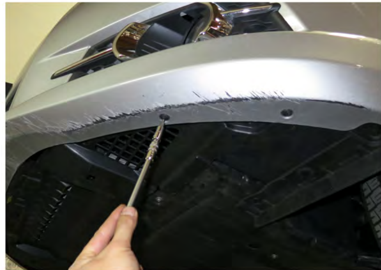
34. Tighten the (8) T20 screws Please repeat the steps from 1 to 34 for the opposite side
