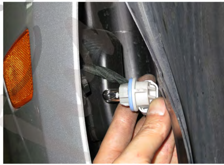
32. Replace the bumper light socket
