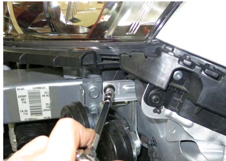
16. Remove the 7mm bolt
