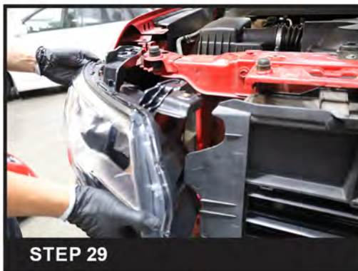
STEP 29 Install the new headlight
