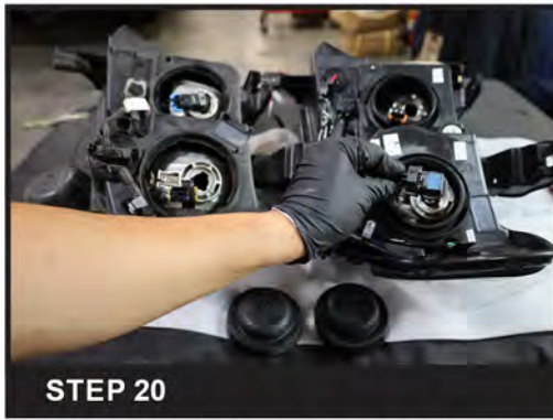
STEP 20 Install the Low beam bulb onto the new headlight
