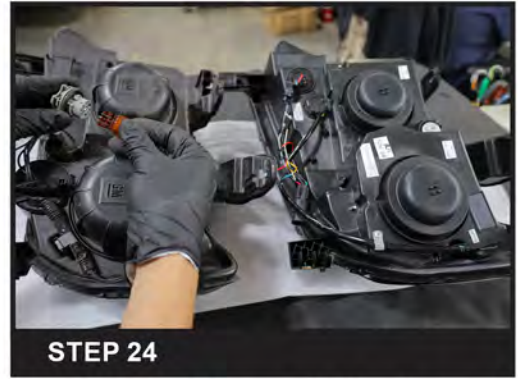
STEP 24 Remove the turn signal bulb from the factory light
