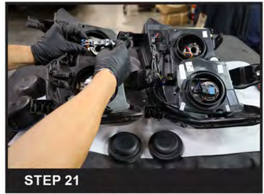
STEP 21 Remove the Hi beam bulb from the factory headlight
