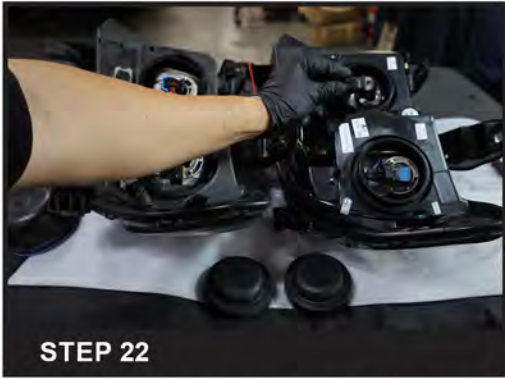
STEP 22 Install the Hi beam bulb onto the new headlight
