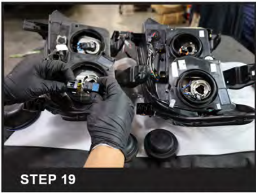
STEP 19 Remove the Low beam bulb from the factory headlight
