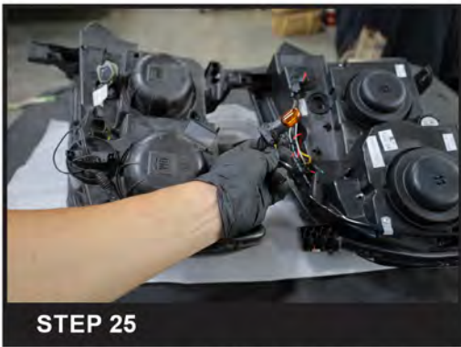
STEP 25 Install the turn signal bulb onto the new headlight socket
