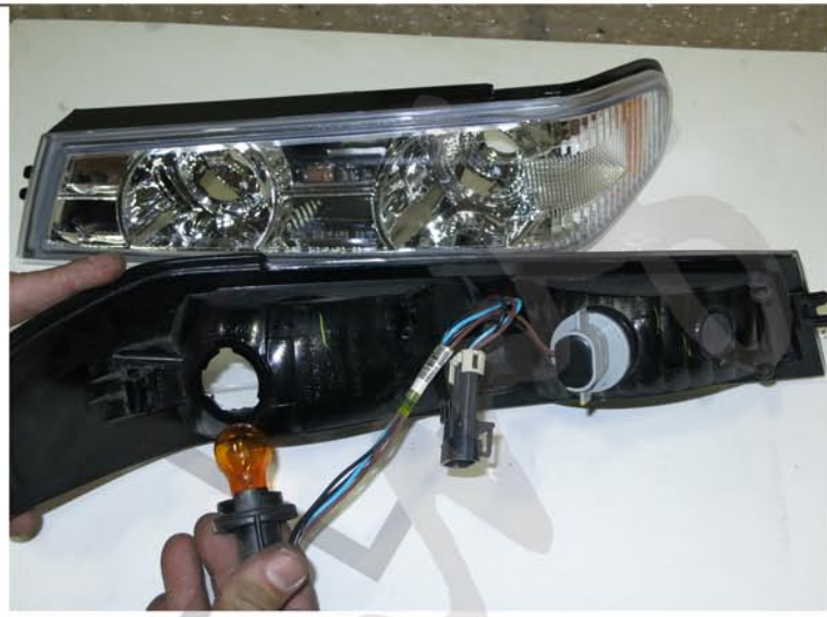
6. Transfer the bumper light harness to the new bumper light
