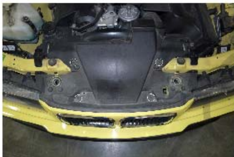
1. (4) Phillips head screws location
