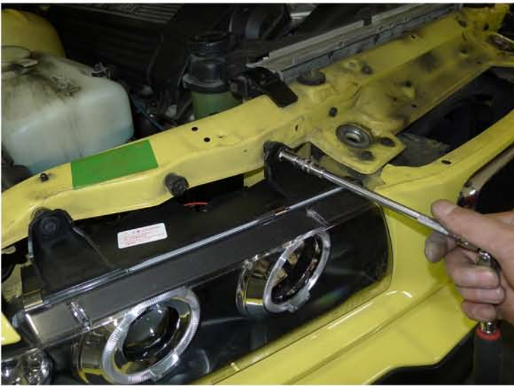
17. Tighten the (3) 8mm bolts
