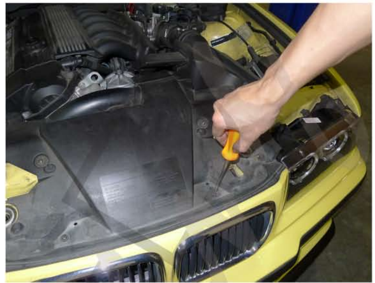
18. Replace the plastic molding and tighten the (4) philips head screws
