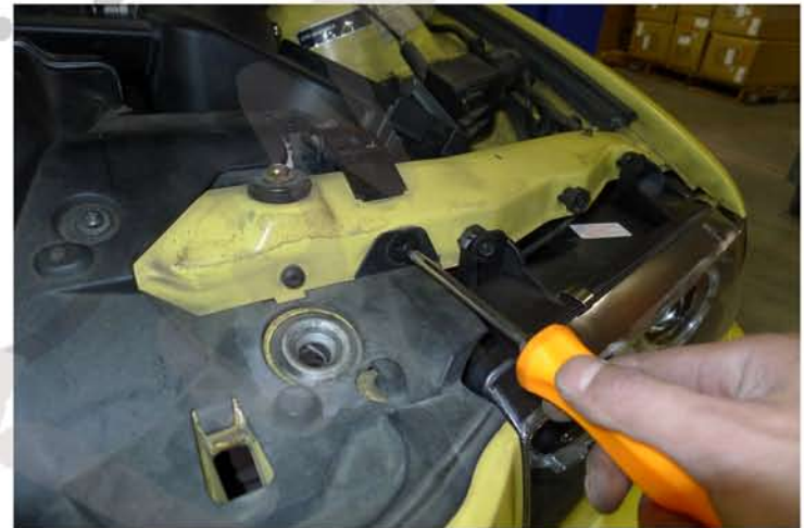
20. Replace the (2) plastic clips
