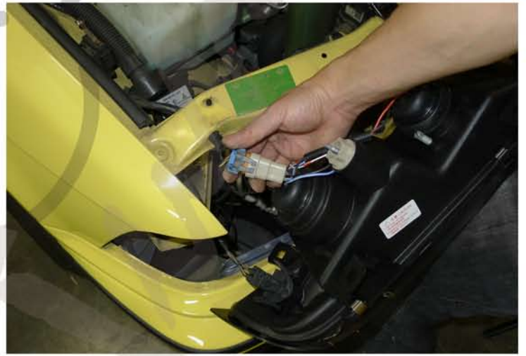
14. Connect the headlight harness to the new headlight Please see the Halo and L.E.D installation instructions If your headlights don't have HALO or L.E.D. You can skip it
